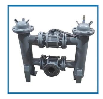
housings. The system also contains a valve handle placed between the two baskets to divert the flow of liquid to one strainer while the other is being cleaned. On some strainers, the valve will work automatically and the strainer will perform a self-cleaning operation. These types of strainers are installed in pipeline systems where flow cannot be stopped.
